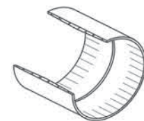
TYPICAL COUPLING FOR PVC PIPE UNDERDRAIN 1/4 SECTION REMOVED
