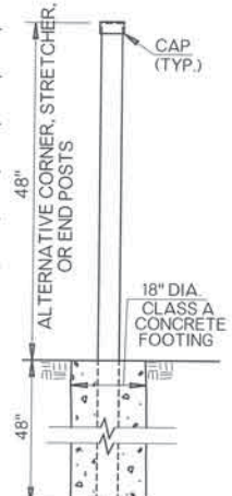
ALTERNATE POST OPTION 3 1/2" DIA. X 8'-0" LG. CAPPED GALV. SCH. 40 STEEL PIPE
