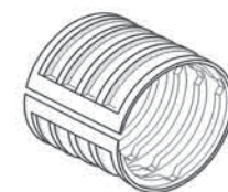
TYPICAL CORRUGATED COUPLING OR AN APPROVED EQUAL
